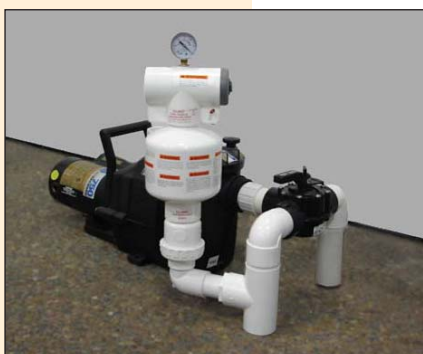
The SVRS is mounted in the main drain suction line, close to the circulation pump.
