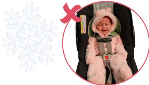
The fluff of a bulky winter coat or snow suit can compress in a car crash making harness straps loose, which can cause injury or ejection.
